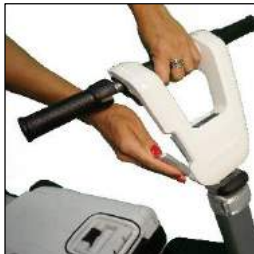
Figure 19 Driving Console tilt lever
