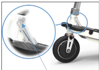
Figure 22 Steering Rod angle adjustment screws
