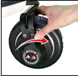
Figure 51 Releasing the freewheel
