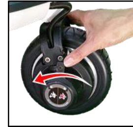
Figure 52 Securing the freewheel
