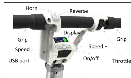
Figure 23 Driving Console overview
