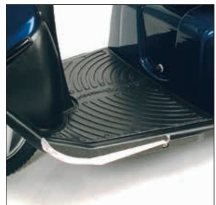
1506-1826 - Extended footplate for 3-wheeler, Right side 1506-1827 - Extended footplate for 3-wheeler, Left side
