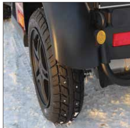
1503-1008 - Wheel, model-X. 2,50-3,70-8" Complete. Black. 6 PR with spikes - Non-Marking.
