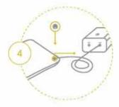
Unscrew the tubing and close the valve cap.
