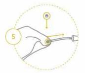
Unscrew the pump hose and screw the safety cap on a valve.
