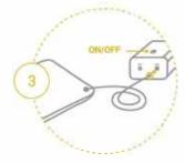
Change the position of hose in the pump from SOFT to HARD and turn it on to suck out the air until the desired hardness is reached.
