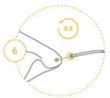
In order to change the shape, screw the hose into a valve, wait until the cushion softens and then repeat points 2 to 5.
