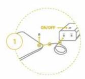
Unscrew the valve cap, screw the threaded part of hose into the cushion valve, press the other part into SOFT socket and turn on the pump. Wait until the cushion is soft enough, then turn off the pump.
